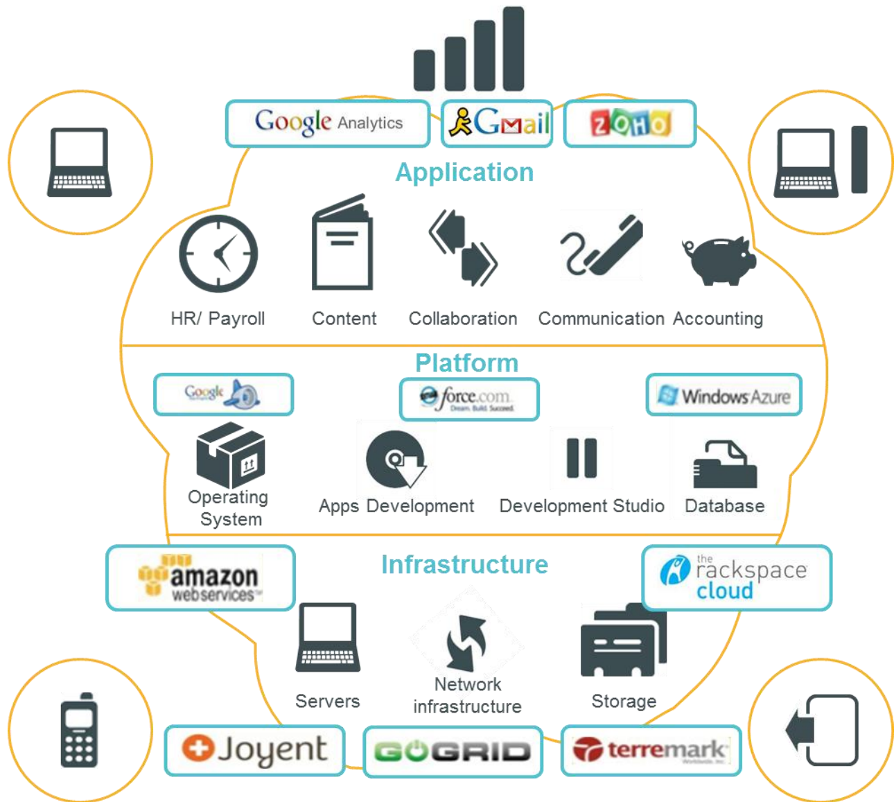
Figure 5: Three types of cloud computing – Application, Platform and Infrastructure as a service
